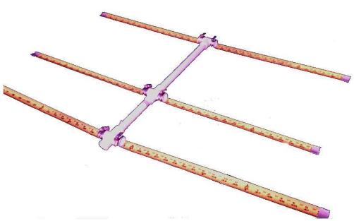
gain, but at the expense of a really good notch in the pattern toward the rear.) It is a design that can be constructed using only simple hand tools (no machine shop needed) and still perform well. It has been duplicated several dozen times by other local hams and has been successfully used as a club construction project.
