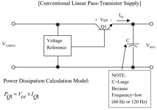
For the conditions:  $V_{UNREG} = 18 \text{ V}$ ;  $V_{REG} = 14 \text{ V}$ ;  $I_{Q1} = 1 \text{ A}$
